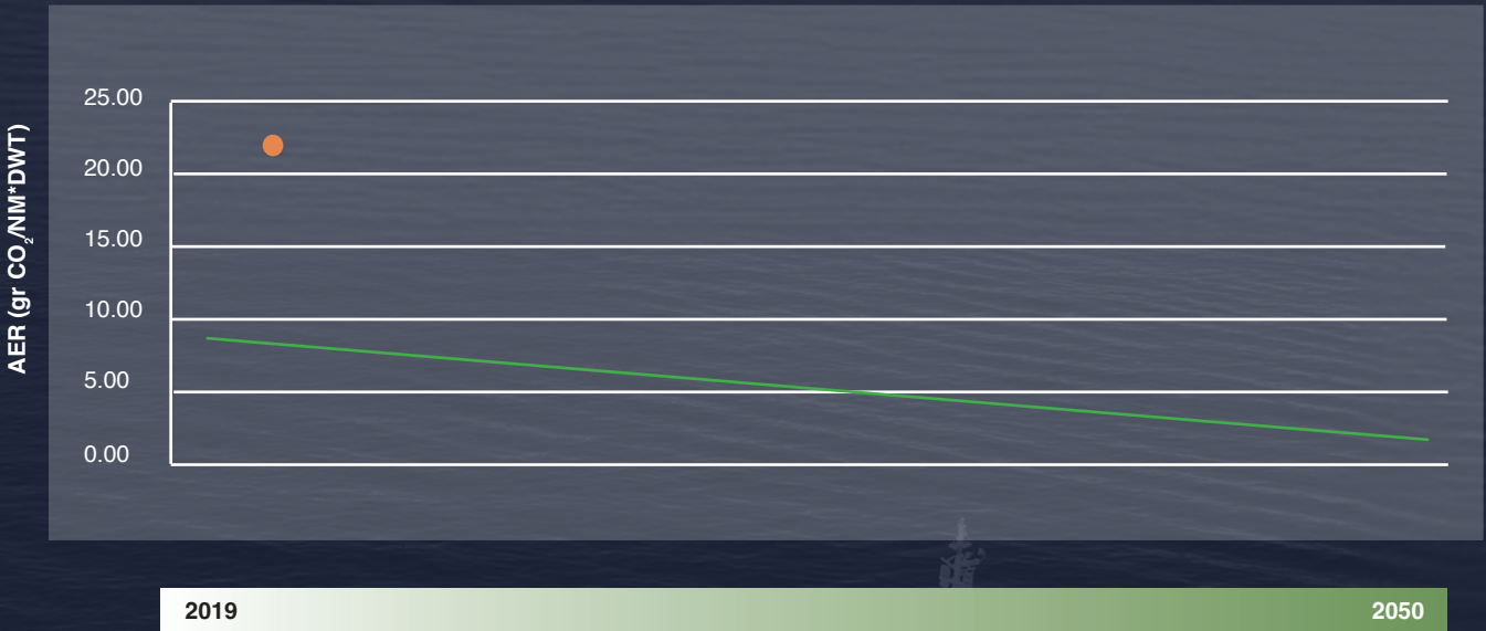
Figure 3. AER Trend for Medium Cement Carriers (10,000-34,999 DWT) Illustrating Carbon Efficiency Improvement from 2019 to 2050, Aligned with Poseidon Principles
