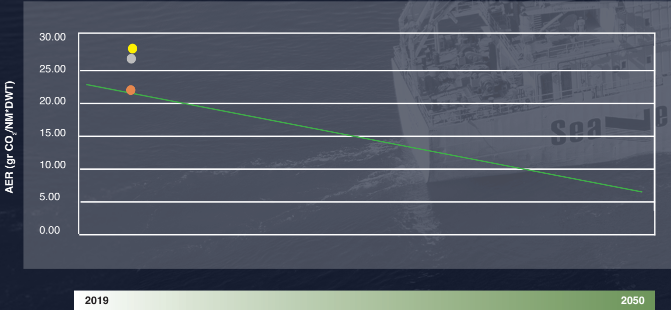
Figure 2. AER for Cement Carriers (DWT<10,000): Projected Decline in Carbon Intensity from 2019 to 2050 in Accordance with Poseidon Principles
