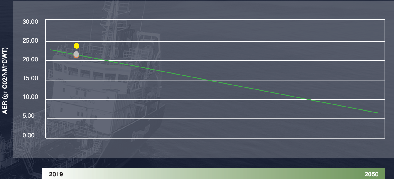
Figure 6. AER Progression for Oil-Chemical Tankers (DWT 5,000 - 9,999): Demonstrating Commitment to Carbon Reduction from 2019 to 2050 in Accordance with Poseidon Principles.
