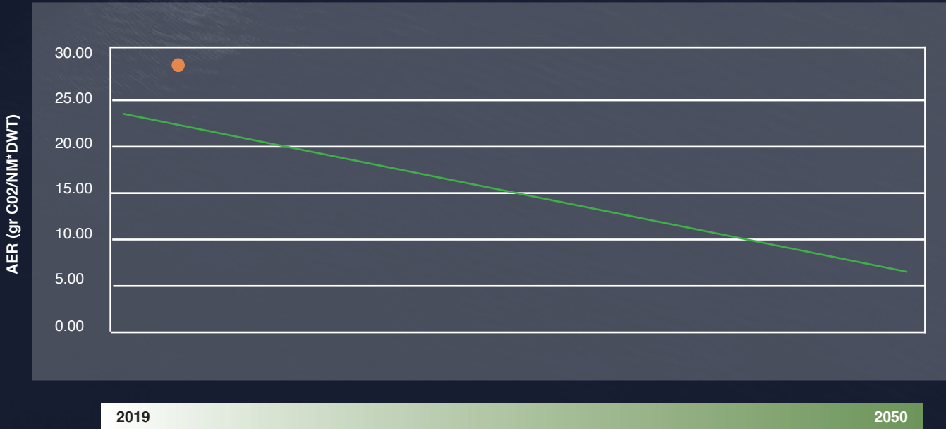
Figure 7. AER Projection for Small to Mid-sized Oil-Chemical Tankers (5,000-9,999 DWT): Charting the Path to Enhanced Carbon Efficiency by 2050 Following Poseidon Principles
